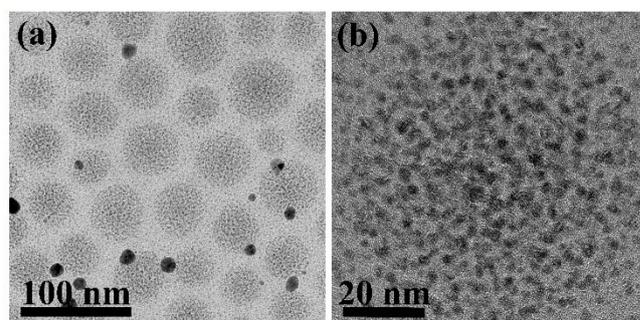
**Fig. 3** (a) TEM image of the Au nanocluster array thin film prepared at 80 °C with 1 h, (b) the corresponding magnified TEM image of the Au cluster.
