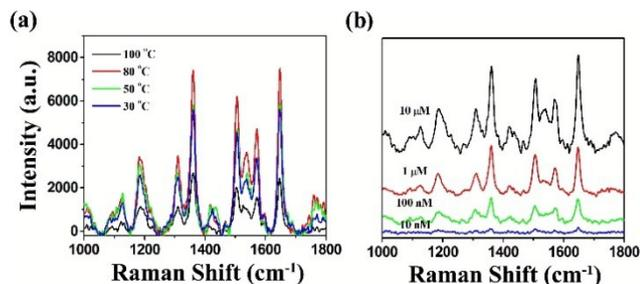
**Fig. 5** (a) SERS spectra of  $10^{-5}$  M R6G methanol solution collected by the Au cluster-like array films prepared at different temperatures. (b) SERS spectra of Au cluster-like array films (prepared at 80 °C) immersed in different concentration of R6G methanol solutions.
