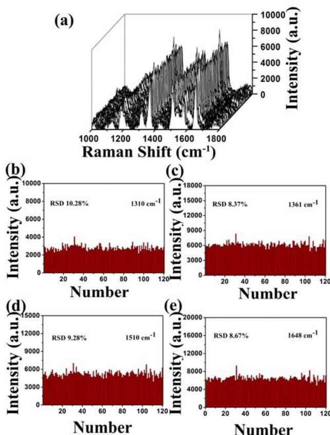
**Fig. 6** (a) Raman scattering spectra of  $10^{-5}$  M R6G measured by 120 points over a  $50 \times 50 \mu\text{m}^2$  area with a step size of 5  $\mu\text{m}$ . (b-e) The intensities of the main Raman vibrations of R6G aqueous solution in SERS spectra showed in (a). A 532 nm excitation laser was used.
