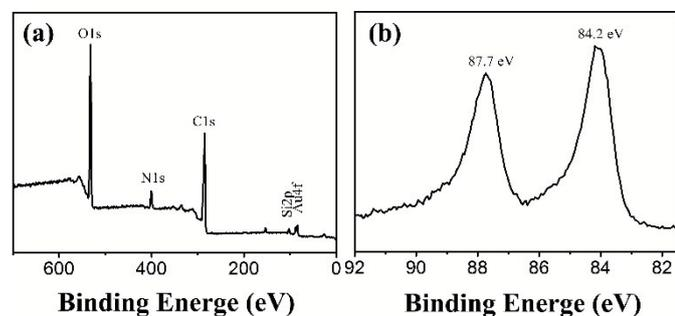
**Fig. 2** (a) XPS spectrum of Au nanocluster array. (b) The high-resolution XPS spectrum of Au 4f.
