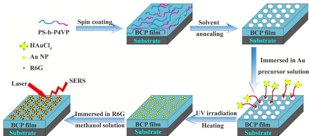
Scheme 1. Schematic illustration for the preparation of Au nanocluster arrays.
