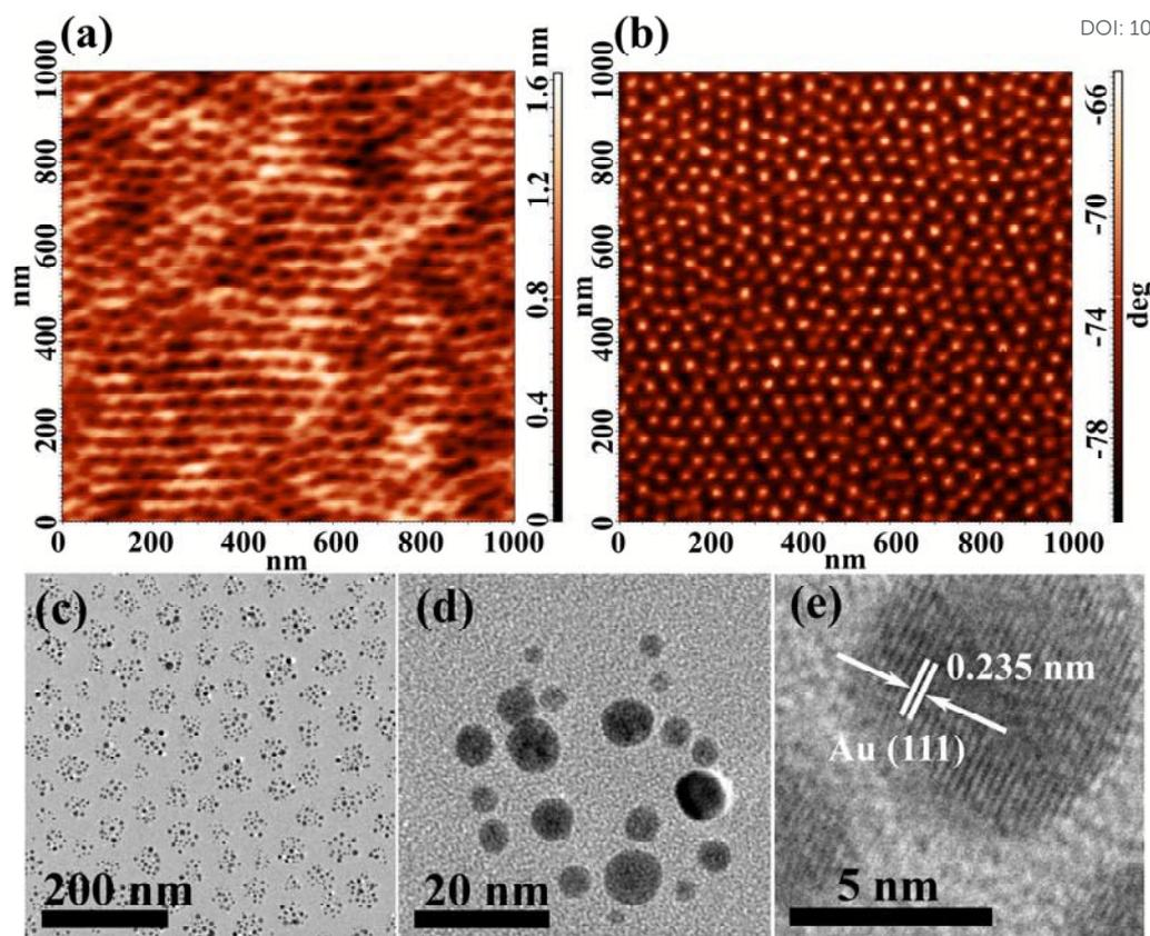
**Fig. 1** AFM height (a) and phase (b) images of self-assembled PS-*b*-P4VP thin film, the scanning size of both images is 1.5 × 1.5 μm<sup>2</sup>. TEM or HRTEM images of (c) Au nanocluster arrays, (d) Au nanocluster, (e) Au nanoparticle prepared at 80 °C with 3 h.
