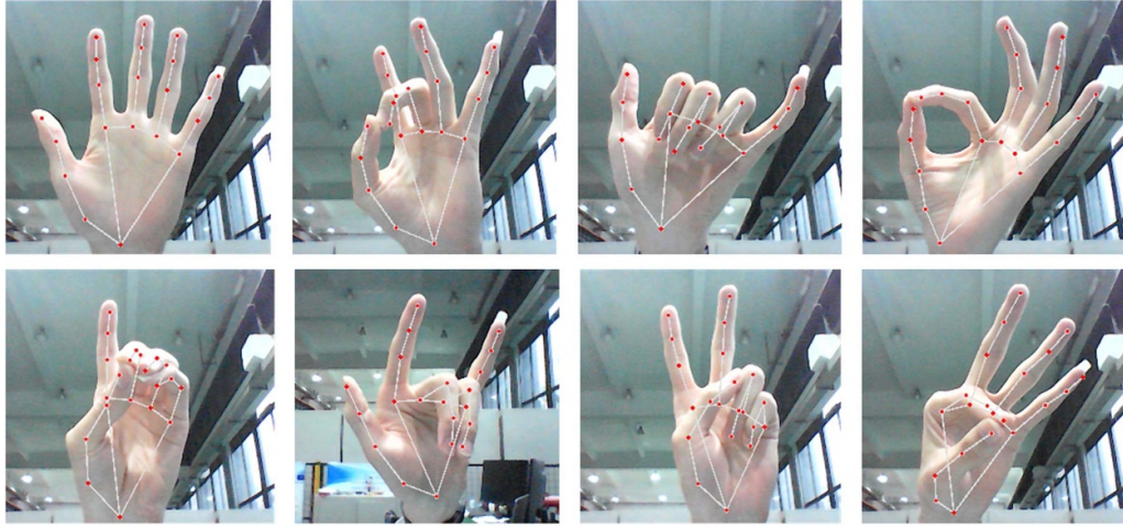
Figure 3. Hand keypoints detected using MediaPipe.
