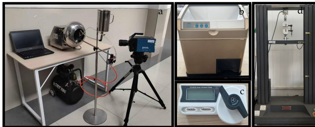
Figure 1. (a) Brown rice humidification experimental platform; (b) rice mill; (c) grain moisture meter; (d) universal tensile tester.
