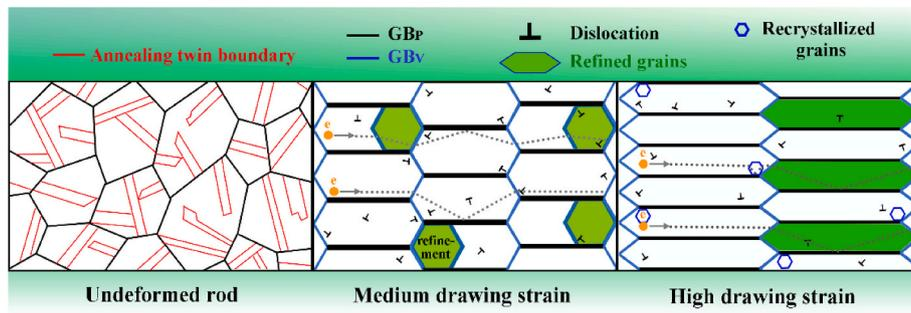
Fig. 10. Schematic diagram of electron scattering by deformed structure.
