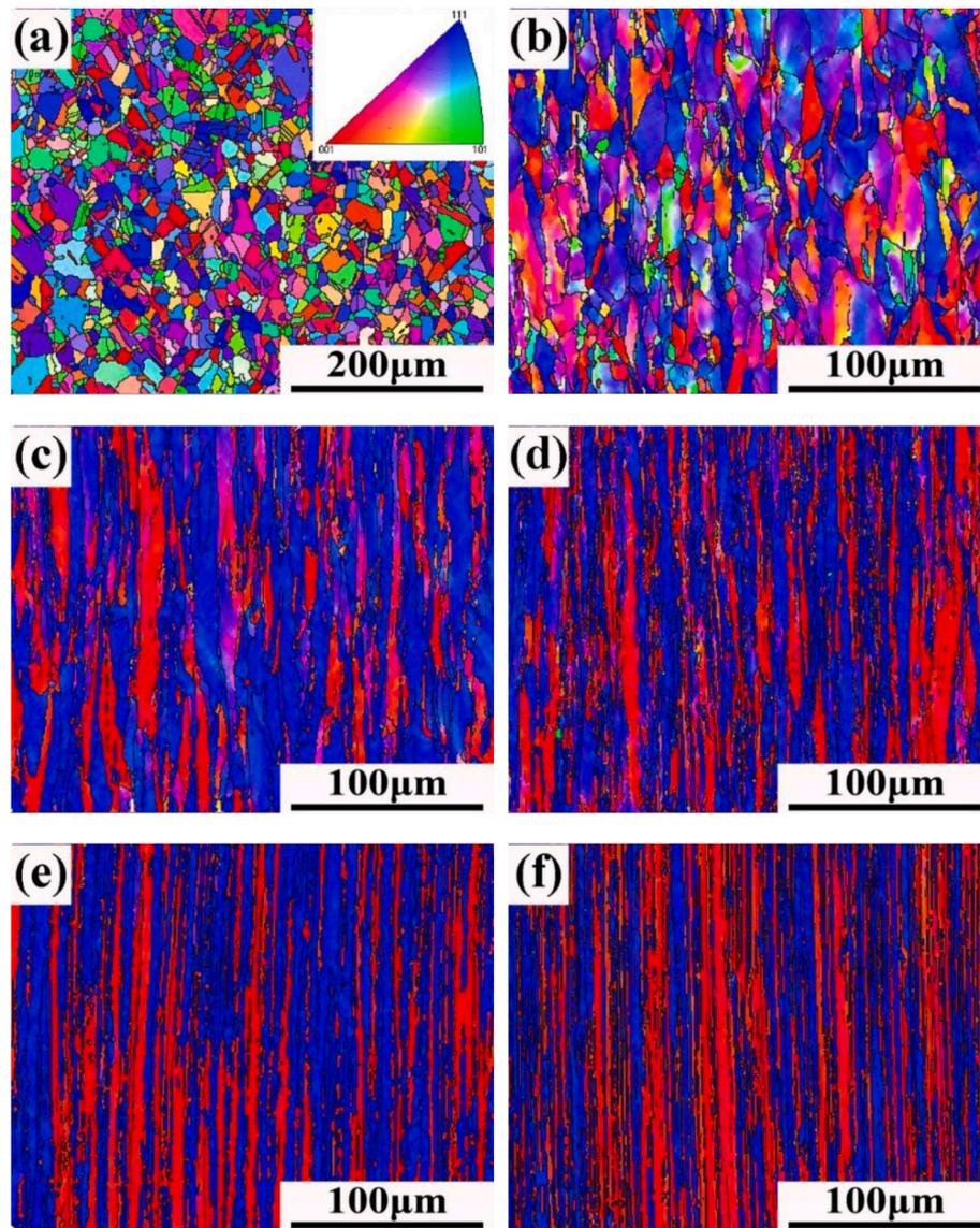
Fig. 3. IPF images in the drawn direction at strains of (a) undeformed, (b)  $\varepsilon = 0.58$ , (c)  $\varepsilon = 1.23$ , (d)  $\varepsilon = 1.91$ , (e)  $\varepsilon = 2.74$ , and (f)  $\varepsilon = 3.47$ .
