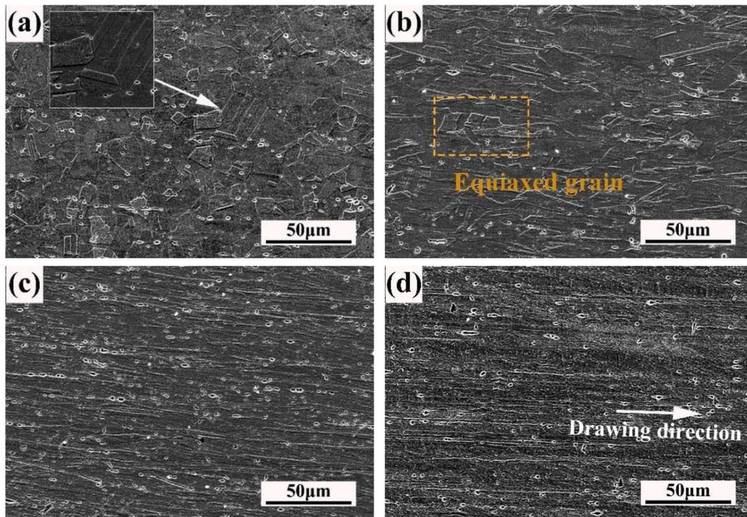
Fig. 1. Microstructure of the longitudinal section with (a) undeformed  $\varepsilon = 0$ , (b)  $\varepsilon = 0.58$ , (c)  $\varepsilon = 1.91$ , and (d)  $\varepsilon = 3.47$ .
