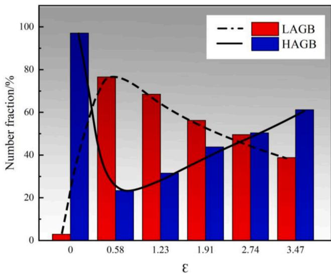
Fig. 5. Misorientation angle variation of cold-drawn copper wires.
