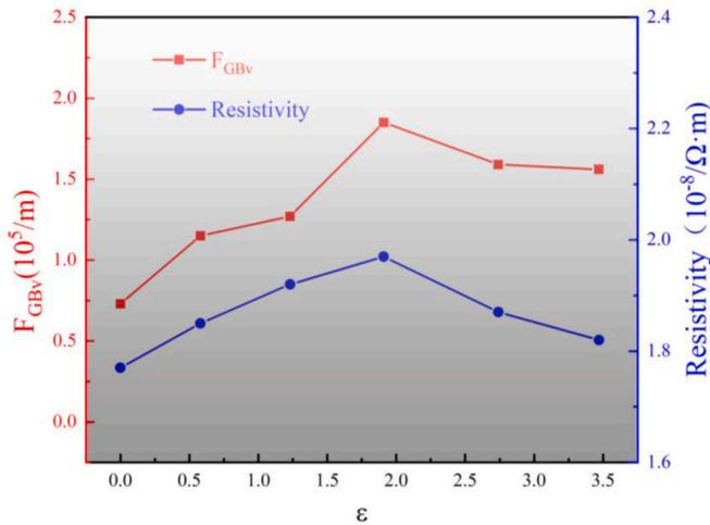
Fig. 11. and resistivity versus drawing strain.
