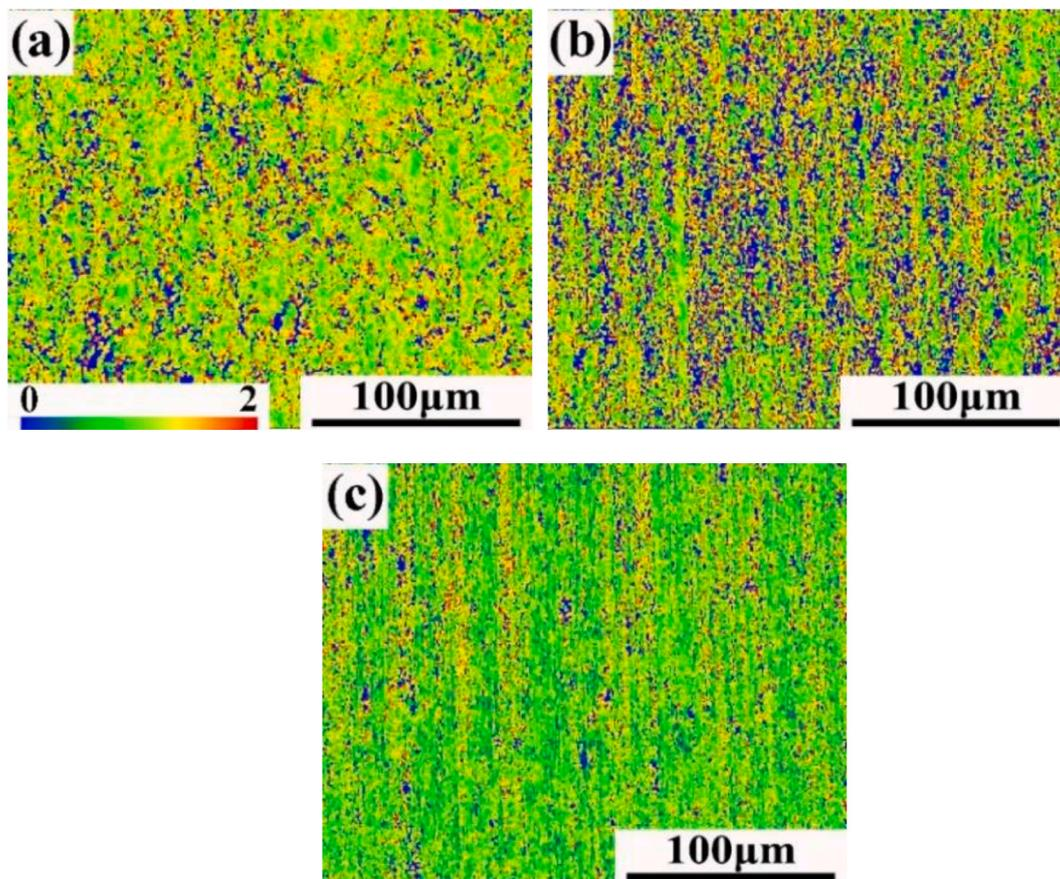
Fig. 4. Kernel average misorientation at strains of (a)  $\epsilon = 0.58$ , (b)  $\epsilon = 1.91$ , and (c)  $\epsilon = 3.47$ .
