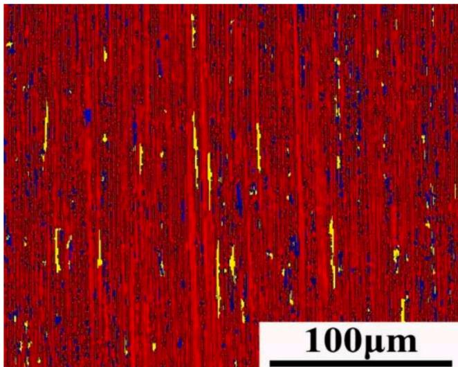
Fig. 12. Recrystallization of copper wire at  $\epsilon = 3.47$ .
