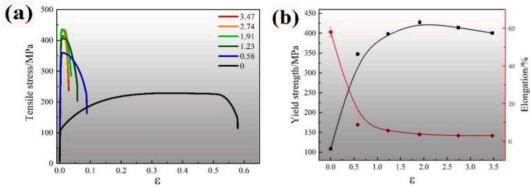
Fig. 6. (a) Engineering stress-strain curves and (b) yield strength and elongation versus drawing strain.
