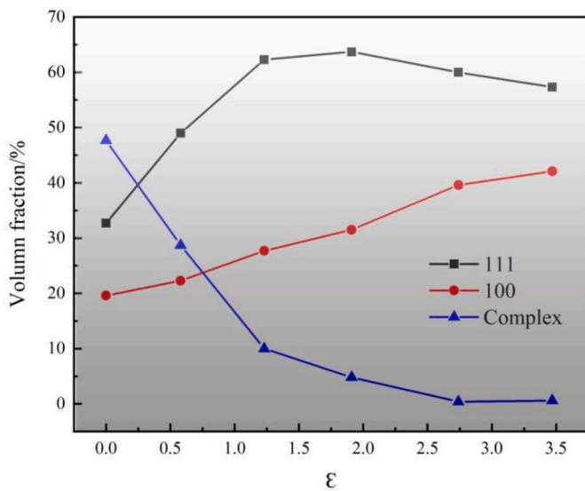
Fig. 8. Variation in the texture components as a function of strain.
