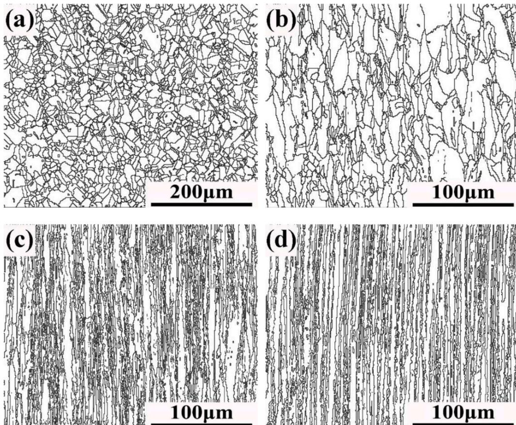
Fig. 9. Distribution of high-angle grain boundaries: (a) undeformed, (b) ε = 0.58, (c) ε = 1.91, and (d) ε = 2.74.
