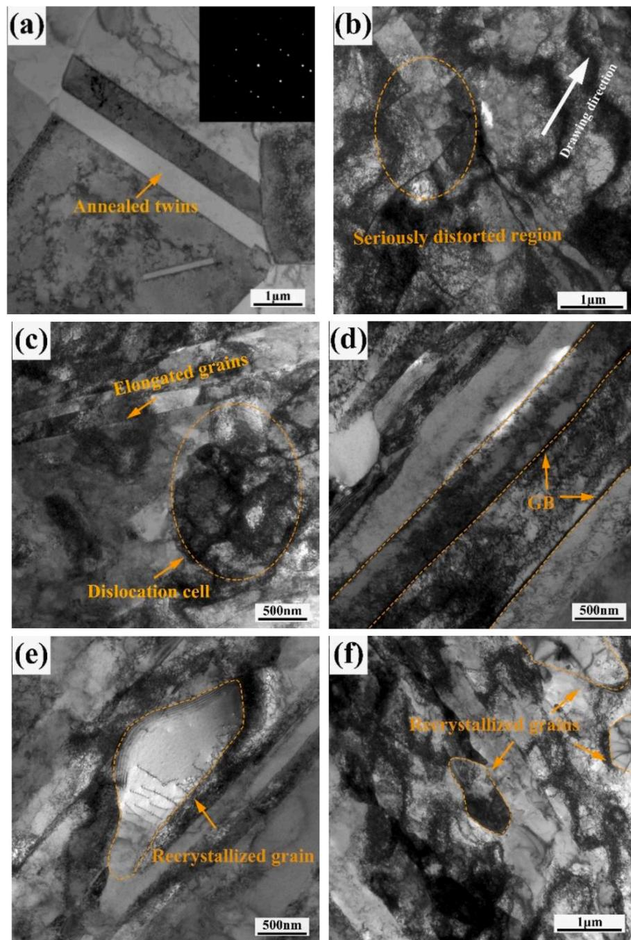
Fig. 2. TEM bright field images at strains of (a) undeformed, (b)  $\epsilon = 0.58$ , (c)  $\epsilon = 1.91$ , (d, e)  $\epsilon = 2.74$ , and (f)  $\epsilon = 3.47$ .
