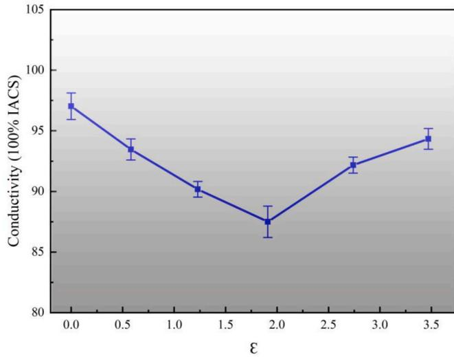
Fig. 7. Conductivity of low-oxygen copper at different strains.
