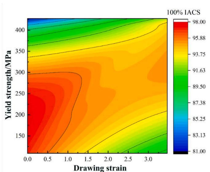
Fig. 13. Electrical conductivity versus drawing strain and yield strength.
