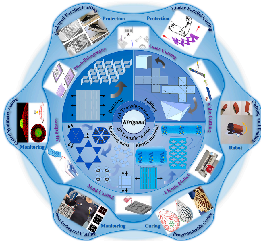
Fig. 1. The Overview of the induced mechanisms, pattern preparation methods and applications of kirigami metamaterials. Inner circle: 2D/3D induced deformation mechanisms of kirigami. Middle circle: preparation methods of different kirigami patterns, including tool cutting, mold casting, 3D printing, photolithography, laser cutting, etc. Reproduced with permission [58]. Copyright 2020, IEEE. Reproduced with permission [59]. Copyright 2023, The Authors. Reproduced with permission [60]. Copyright 2023, AIP Publishing. Reproduced with permission [61]. Copyright 2023, Wiley. Reproduced with permission [62]. Copyright 2020, American Chemical Society. Reproduced with permission [63]. Copyright 2019, American Chemical Society. Outer circle: current and potential applications of different kirigami shapes in the medical field, including protection, monitoring, curing, soft robots, etc. Reproduced with permission [21]. Copyright 2020, Springer Nature. Reproduced with permission [64]. Copyright 2024, Elsevier. Reproduced with permission [26]. Copyright 2024, Elsevier. Reproduced with permission [65]. Copyright 2024, The Authors. Reproduced with permission [18]. Copyright 2022, Wiley. Reproduced with permission [66]. Copyright 2019, The Authors.
