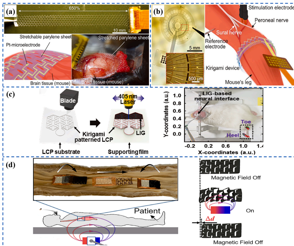
Fig. 11. Kirigami-based implantable health monitoring devices. (a) The design of the bio-probe with parallel linear cutting pattern and its monitoring ECoG signals from the mouse. Reproduced with permission [204]. Copyright 2017, Wiley. (b) The design of the doughnut-shaped kirigami probe and its monitoring of EMG signals from the mouse hindlimb. Reproduced with permission [205]. Copyright 2019, Wiley. (c) The design of the electrode patch with the Y-shaped cutting pattern and its monitoring of sensory signals from mouse tactile stimulation. Reproduced with permission [206]. Copyright 2023, The Authors. (d) The intervention device integrating a kirigami soft robot and sensor for wireless monitoring of GERD, and the movement form of the soft robot. Reproduced with permission [85]. Copyright 2023, American Chemical Society.
